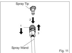
1-Pull back the quick-connect collar 2-Push the spray tip into place
